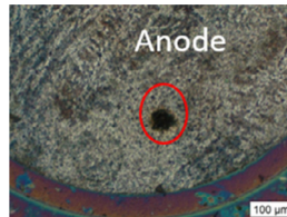
Fig. 7. Optical Microscopy after high voltage failure.
