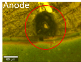
Fig. 8. Optical microscopy after high voltage failure on the corner of the device.
