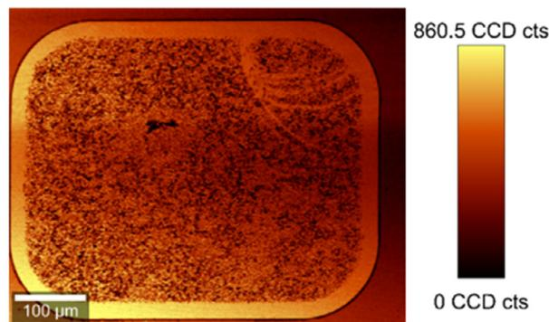
Fig. 19. Micro-Raman mapping of the Sic integrated intensity.
