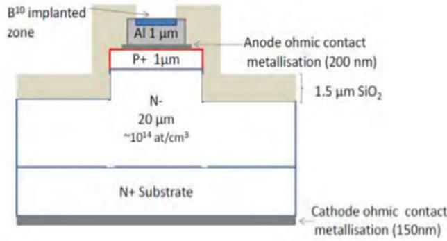
Fig. 1. Transversal section of vertical SiC diode.
