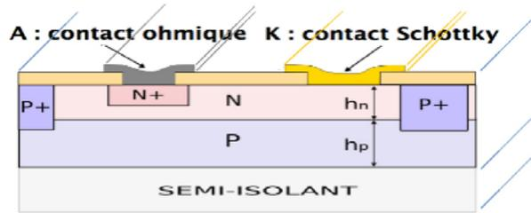
Fig. 2. Transversal section of lateral Schottky diode.
