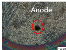
Fig. 7. Optical Microscopy after high voltage failure.
