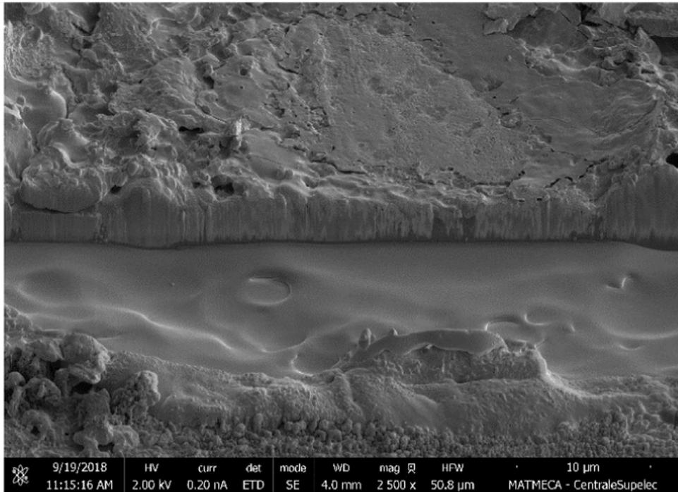
Fig. 15. Zoom on failure in SiC vertical diode.
