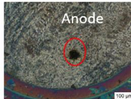
Fig. 7. Optical Microscopy after high voltage failure.
