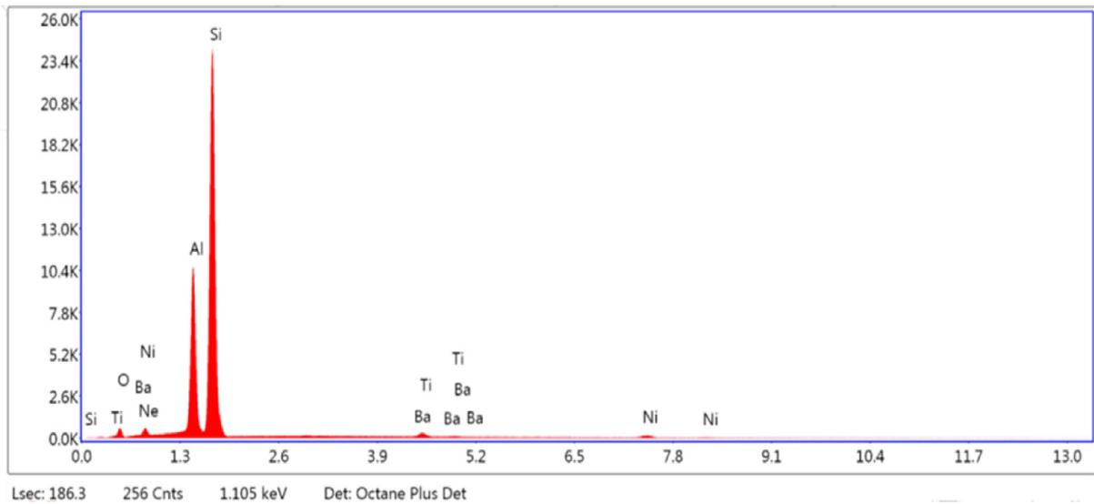
Fig. 17. EDX of SiC vertical diode before failure.
