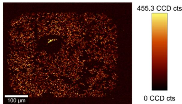
Fig. 18. EDX of Sic vertical diode after failure.
