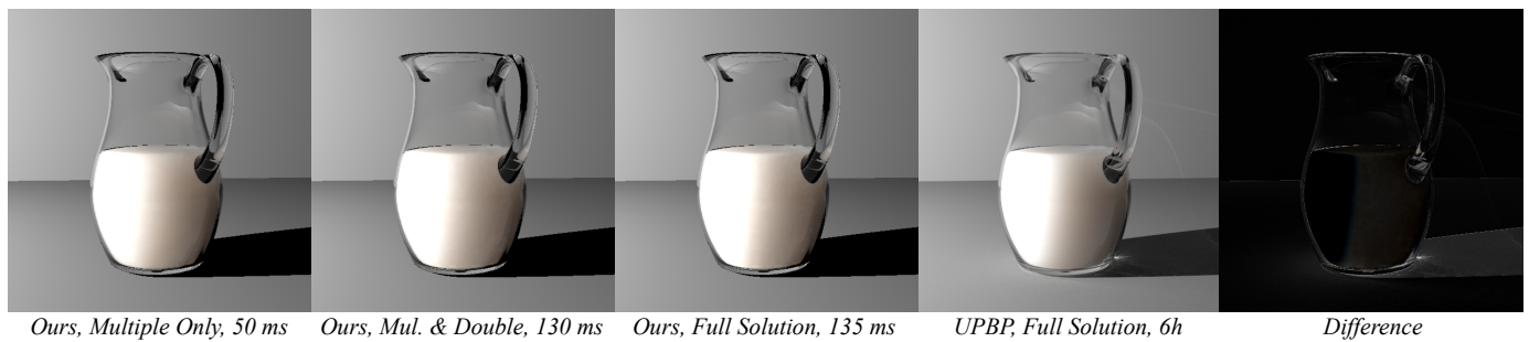
Fig. 9. With high-albedo, small mean-free path materials like milk, our algorithm produces images that are very close to the reference, at a fraction of the cost. It should be noted here that GPU ray-tracing does not handle transparency effects, which causes the difference in shadows. Material: Milk.
