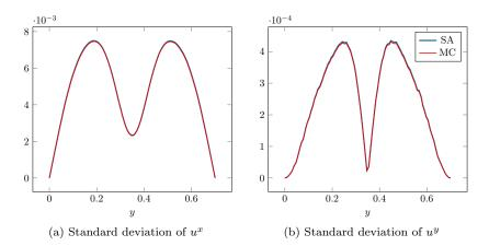
Figure 7: Standard deviation on the vertical cross section x = 1. Comparison between Monte Carlo and the SA estimate.
