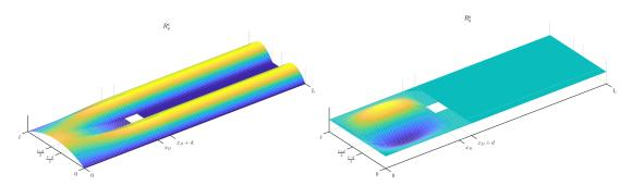
Figure 17: Solenoidal field from the example, x and y components.
