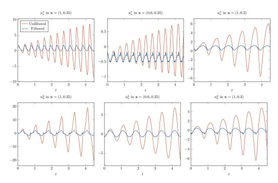
Figure 14: Filter applied to the sensitivity of the velocity in three different points of the domain. Top row: horizontal component. Bottom row: vertical component.
