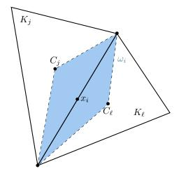
Figure 2: The control volume  $\omega_i$  associated with the node  $\mathbf{x}_i$  is shaded in blue.  $C_j$  and  $C_\ell$  are the centres of gravity of the two triangles  $K_j$  and  $K_\ell$  adjacent to the edge on which  $\mathbf{x}_i$  lies.
