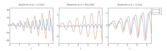
Figure 11: Sensitivity of the velocity field in three different points of the domain with respect to time.
