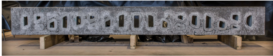
(b) Demoulding of the beam
