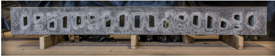
(b) Demoulding of the beam
