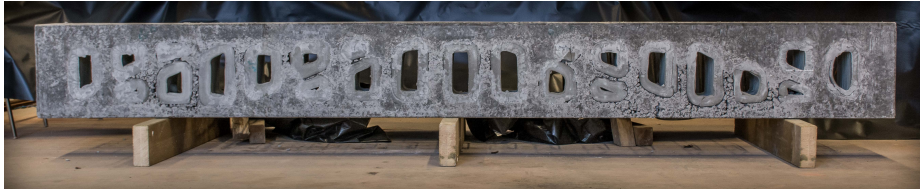
(b) Demoulding of the beam
