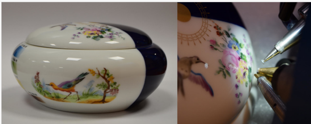
Left, the test object: a glazed porcelain pot with a fine polychrome decoration showing the area to be scanned featuring a tree. Right, the object in the 3D positioner in the external beam end-station.
