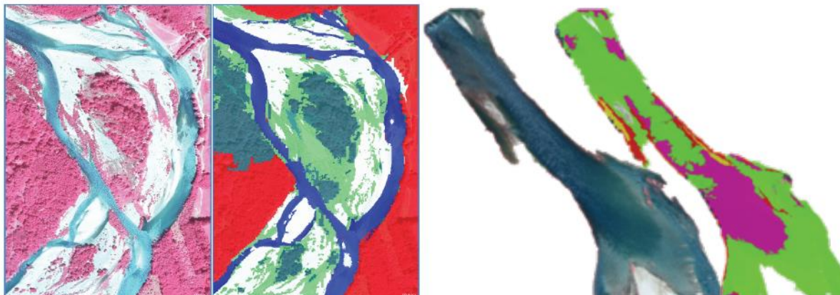
Figure 8. Workflow of the multilevel, object-based methodology developed for the classification of riverscape units and in-stream mesohabitats. Top row shows data type used (multispectral and Lidar derived DTM); central row describes the OBIA steps to derive topographically and spectrally homogenous units; the bottom row displays classification results for riverscape units (on the left) and mesohabitats (on the right). (Source: Demarchi et al. 2016 Figure 5)
