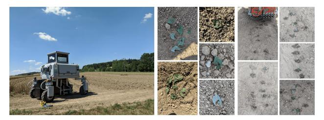
Figure 14: Left: example picture of field robot performing weed control evaluation. Middle: sample pictures of leaves after mechanical weed removal. Right: sample pictures after selective spraying.
