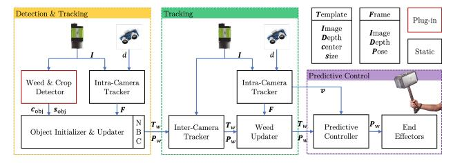
Figure 5: An overview of our proposed weed control system that is composed of weed detection, tracking and predictive control modules. The symbols used in the figure is briefly explained in upper-right corner.
