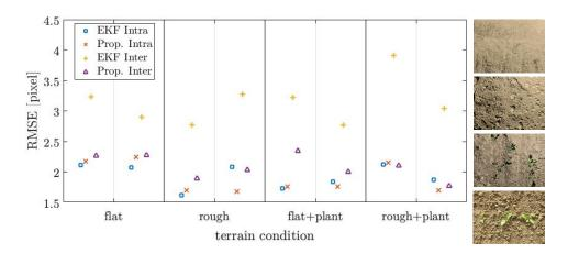
Figure 12: Tracking accuracy analysis on effect of terrain conditions using Renningen Dataset. Left: the intraand inter-camera tracking RMSE comparison between EKF-based approach and our proposed optimization-based approach versus test sequences with different terrain conditions. Right: Example images acquired in four typical real field condition (Top-to-Bottom): flat surface, rough surface, flat surface with plants, and rough surface with plants.
