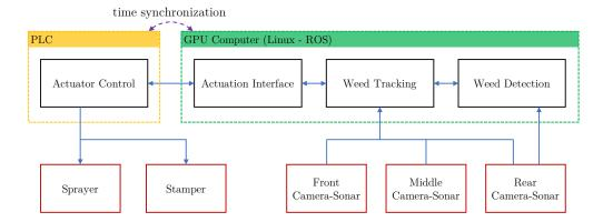
Figure 3: Architecture of computers, sensors and actuators dedicated to the weed treatment.
