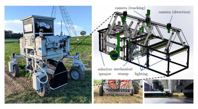
Figure 2: Left: the robotic platform Flourish BoniRob with our proposed weed control unit mounted at the bottom. Upper-Right: a CAD view of the unit including the actuators and sensors. Bottom-Right: the pictures of the selective sprayer and the mechanical stamping tool.
