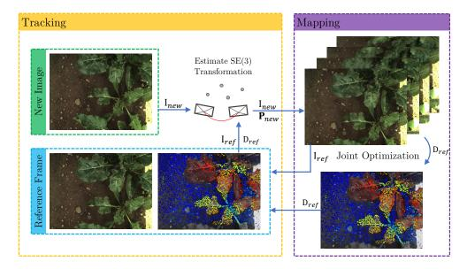
Figure 8: The overview of our proposed intra-camera tracking and mapping algorithm.
