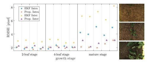
Figure 11: Tracking accuracy analysis on effect of different crop growth stages using Ancona and Zurich Dataset. Left: the intra- and inter-camera tracking RMSE comparison between EKF-based approach and our proposed optimization-based approach are versus test sequences with different crop growth stages. Right: Example images acquired in four typical real field condition (Top-to-Bottom): flat surface, rough surface, flat surface with plants, and rough surface with plants.
