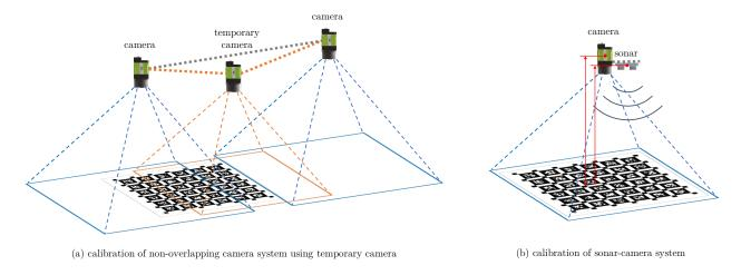
Figure 4: The schematic of sensor calibration. Left: the calibration of non-overlapping cameras using overlapping calibration software by introducing assistant camera in between. Right: the calibration of the camera and sonar height difference uses a marker field perpendicular to the central axes of the sensors.
