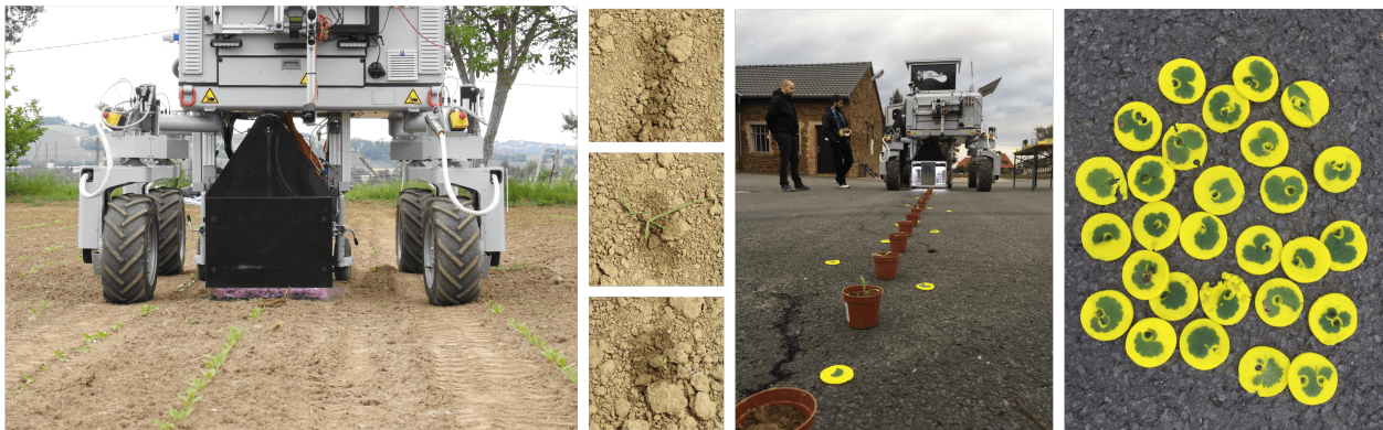
Figure 15: Left: an in-row selective spraying test is conducted in real-world field in Ancona (Italy), where the marks after spraying can be clearly seen in the picture. Right: the performance of in-row mechanical weeding is presented in simulated test environment in Bonn (Germany), where the faked targets made of leaves attached on modeling clay is used to visualize the execution results.
