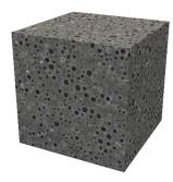
Figure 2: Tomography image of composite with 30%vol HGM
