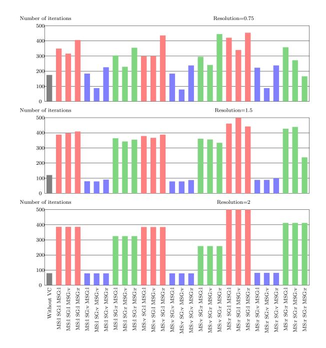
Figure 7: Histogram plot of number of iterations as a fonction of all combinations of composite voxels homogenization rules for the resolution of 0.75, 1.5 and 2 and for the reference matrix properties (i.e. shell/matrix elastic contrast = 63).
