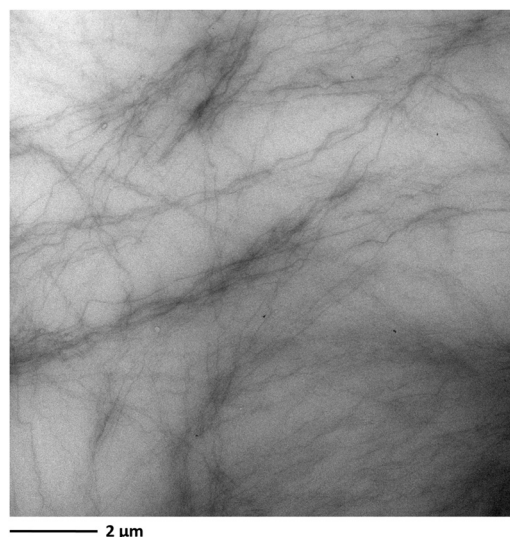
Fig. 2 TEM micrograph of the organogel after negative staining.
