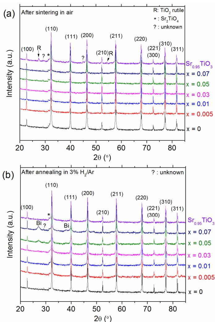
Fig. 1 X-ray diffraction patterns of  $\text{Sr}_{1-x}\text{Bi}_x\text{TiO}_{3-\delta}$  ( $x = 0, 0.005, 0.01, 0.03, 0.05,$  and  $0.07$ ) and  $\text{Sr}_{0.95}\text{TiO}_{3-\delta}$  ceramics (a) after sintering in air and (b) after annealing in a reducing atmosphere. Letter R, star (\*), question mark (?), and Bi indicate diffraction peaks corresponding to rutile  $\text{TiO}_2$ ,  $\text{Sr}_2\text{TiO}_4$ , unknown phases and Bi metal, respectively.
