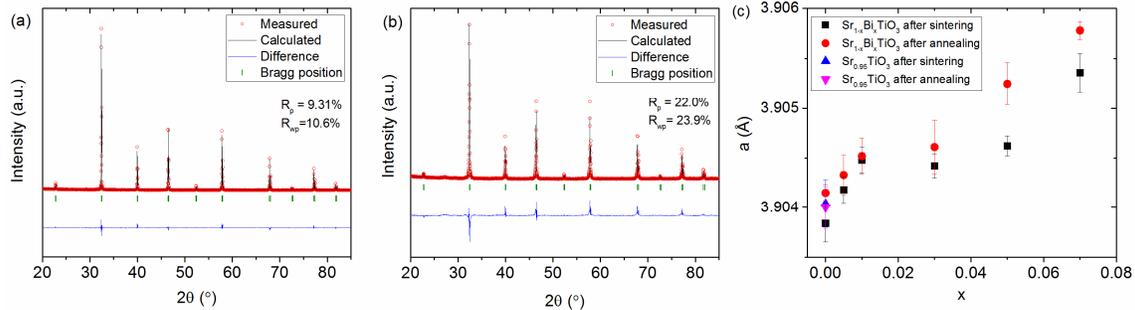
Fig. 2 Examples of Rietveld refinement of  $\text{Sr}_{1-x}\text{Bi}_x\text{TiO}_{3-\delta}$  ceramics after annealing in a reducing atmosphere with a composition (a)  $x = 0$  and (b)  $x = 0.05$ . (c) Lattice parameter  $a$  of  $\text{Sr}_{1-x}\text{Bi}_x\text{TiO}_{3-\delta}$  ( $x = 0, 0.005, 0.01, 0.03, 0.05, \text{ and } 0.07$ ) and  $\text{Sr}_{0.95}\text{TiO}_{3-\delta}$  after sintering in air and after annealing in a reducing atmosphere versus  $x$ .
