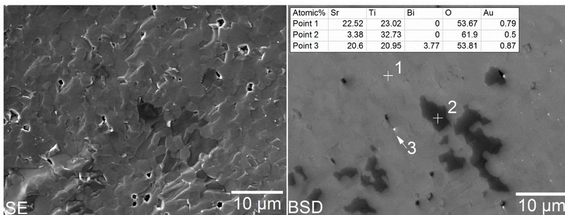
Fig. 3 SEM and BSD images of fracture surface of  $\text{Sr}_{1-x}\text{Bi}_x\text{TiO}_{3-\delta}$  with  $x = 0.01$  after annealing in a reducing atmosphere. The insert in the BSD image shows the atomic ratio of elements at three indicated points measured by EDS.
