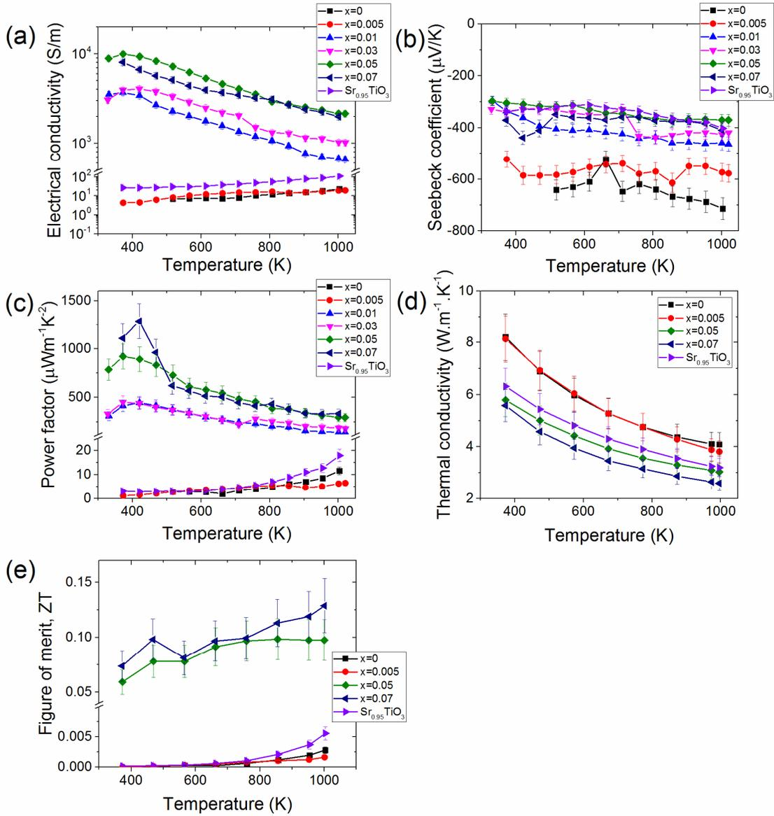
Fig. 4 Thermoelectric properties of  $\text{Sr}_{1-x}\text{Bi}_x\text{TiO}_{3-\delta}$  ( $x = 0.005, 0.01, 0.03, 0.05,$  and  $0.07$ ) and  $\text{Sr}_{0.95}\text{TiO}_{3-\delta}$  ceramics after annealing in a reducing atmosphere as a function of temperature. (a) Electrical conductivity, (b) Seebeck coefficient, (c) power factor, (d) thermal conductivity, and (e) figure of merit,  $ZT$ .
