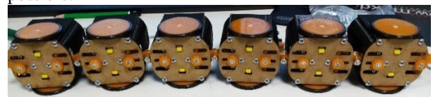
Fig. 5. The orange screw allows the tuning of distance of the different wagons but also the angle for the movement.
