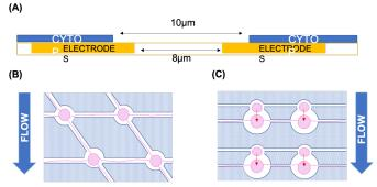
Figure 5. (A) Transversal view of CYTOP wells on ITO glass. (B) Designed channels for 4 possible guided axonal extensions. (C) bi-directional axonal projection with larger well at the bottom of smaller cell trapping well for spatial growth
