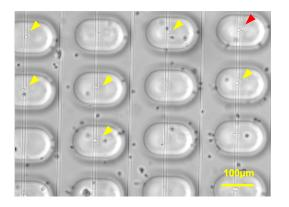
Figure 4. Primary neurons inside trap and drop device. Yellow arrows show single neural cells trapped in one well. Red arrow shows two different neuron cell sizes trapped in a well.
