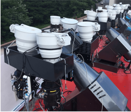
Figure 1. The GWAC telescope network at the Xinglong Observatory in China. Currently, 4 mounts are operational among 10 at completion. Each mount is equipped with four JFoV cameras (18 cm) and one FFoV camera (3.5 cm) located at the centre of the mount. The total FoV of the current GWAC network is about 2000 deg 2 .
