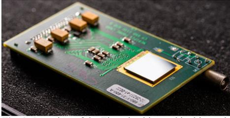
Fig. 1. Overview of the Timepix chip used in this work.
