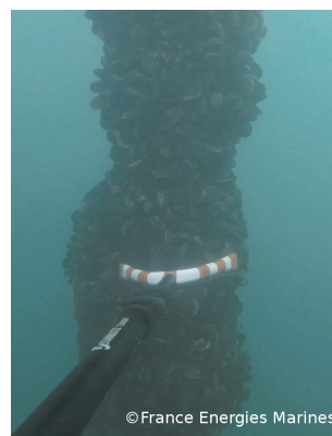
Figure 4. Photograph of bio-colonisation on East cardinal buoy mooring chain of the SEMREV test site in February 2018.
