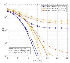
Fig. 3: BER performance of different APM-GSM systems with sub-THz impairments. The spectral efficiency is 12bpcu and both systems are subjected to phase noise with different levels using DO setup. The concerned sub-THz indoor MIMO channels are generated using URA array geometry with  $4\lambda$  antenna separation and  $N_r=10$ . The AP-MS distance is d=[2m,8m] with  $d_{mean}=5m$ .
