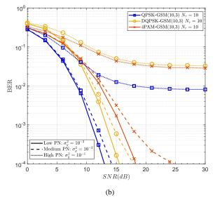
Fig. 2: BER performance of different APM-GSM systems with sub-THz impairments. The spectral efficiency is 12bpcu and both systems are subjected to phase noise with different levels using DO setup. The concerned sub-THz indoor MIMO channels are generated using ULA array geometry with  $4\lambda$  antenna separation. The AP-MS distance is  $d=[2m,\,8m]$  with  $d_{mean}=5m$ . (a)  $N_r=6$ , (b)  $N_r=10$ .
