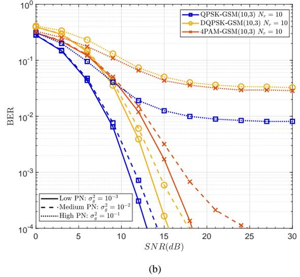
**Fig. 2:** BER performance of different APM-GSM systems with sub-THz impairments. The spectral efficiency is 12bpsu and both systems are subjected to phase noise with different levels using DO setup. The concerned sub-THz indoor MIMO channels are generated using ULA array geometry with  $4\lambda$  antenna separation. The AP-MS distance is  $d = [2m, 8m]$  with  $d_{mean} = 5m$ . (a)  $N_r = 6$ , (b)  $N_r = 10$ .
