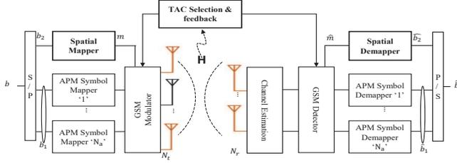
Fig. 1: System model of GSM with TAC selection
