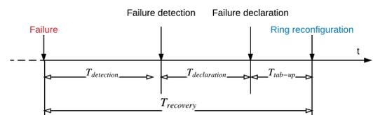
Fig. 7. Recovery time since the failure occurrence until the ring reconfiguration
