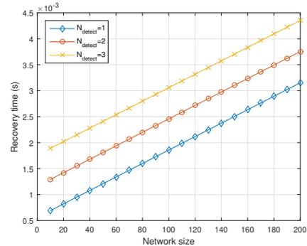
Fig. 10. The impact of  $N_{detect}$  on the Maximum Recovery Time vs the Network Size for ( $M \in [10 : 10 : 200]$ ,  $N_{detect} \in [1 : 1 : 3]$ ,  $P_{local\_detect} = high$ )
