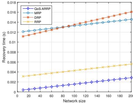
Fig. 12. Recovery time for the different Redundancy Protocols
