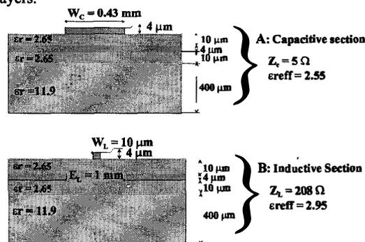
Fig. 1. Technology Si-BCB; capacitive and inductive sections.
