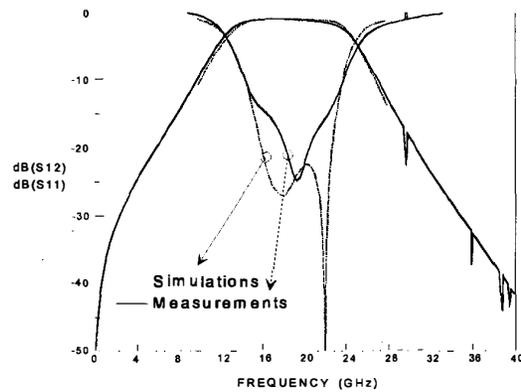
Fig. 8. Experimental and simulated responses in the in-band.
