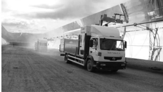
Figure 7: ELCOS Vehicle for pressurised water-cleaning of solar mirrors
