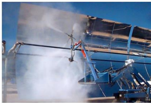
Figure 2: High-pressure, low water volume, with rotating head rig system
