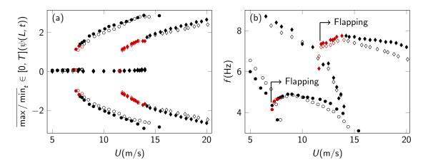
Figure 4 – Experimental results for inverted flags with L = H = 160 mm and  $[\bullet] h = 0.76 \text{ mm}$ ,  $[\bullet] h = 1.02 \text{ mm}$ ; (a) bifurcation diagram (b) variation of the dominant frequency in PSD with the flow speed. The empty and filled markers correspond to the flags with and without the splitter plate, respectively; the black and red symbols correspond to the wind speed sweep up and down, respectively.
