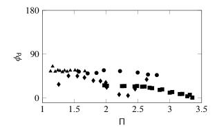
Figure 10 – Phase difference between transverse force (lift) and transverse displacement for stainless steel inverted flags with  $[\blacksquare] L = 100 \text{ mm}$ ,  $[\bullet] L = 70 \text{ mm}$ ,  $[\bullet] L = 50 \text{ mm}$ , and  $[\blacktriangle] L = 35 \text{ mm}$  over the periodic large-amplitude flapping regime.
