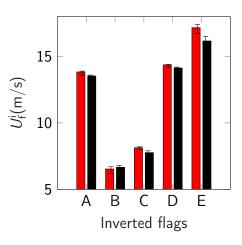
Figure 5 – Critical flow speed for the onset of large-amplitude flapping of different inverted flags with sweeping up the wind speed; [ $\blacksquare$ ] with and [ $\blacksquare$ ] without the rigid splitter plate.
