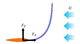
Figure 7 – Measured forces at the flagpole, utilizing a force balance.
