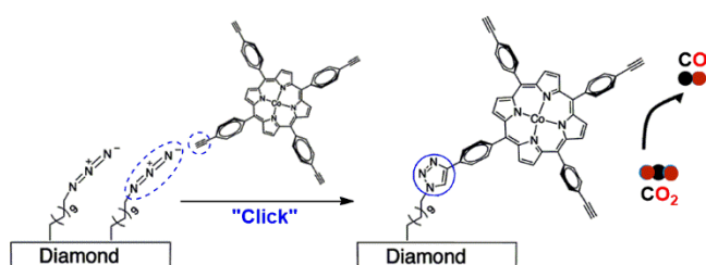
Figure 15. Covalent modification of a diamond cathode surface for the heterogeneous electrocatalytic CO 2 reduction. Adapted with permission from Ref. 83.
