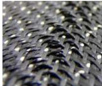
Figure 2: “buckles” mesoscopic defect.
