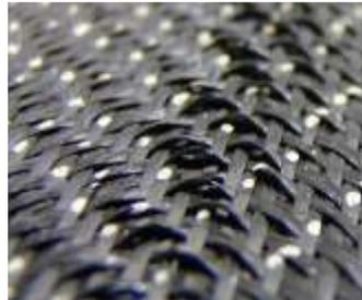
Figure 2: “buckles” mesoscopic defect.
