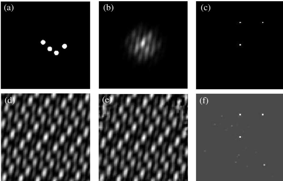
**Fig. 10.** Image reconstruction simulation for the VLTI/VIDA instrumental setup. (a): VLTI pupil. (b): interferometric image of the test object. (c): test object (triple star). (d): theoretical PSF. (e): Reconstructed PSF after 50 000 iterations. (f): Reconstructed object after 50 000 iterations.
