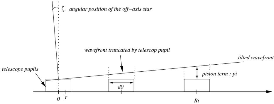
**Fig. 5.** Simulated observation of an off-axis point-source at a distance  $\zeta$  from the center of the field of view. On this one-dimensionnal configuration, each telescope is at a position  $R_i$ . The corresponding complex amplitude on each pupil is the product of a piston term  $\exp 2i\pi\zeta R_i/\lambda$  by a tilt term  $\exp 2i\pi\zeta r/\lambda$ ,  $r$  being the coordinate inside the pupil function.
