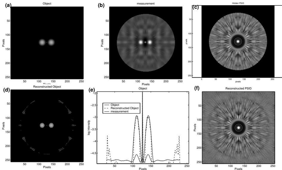
**Fig. 9.** Result of deconvolution for a 39 telescopes interferometer. (a): object; (b): observed blurred image with  $N = 10^{10}$  photons ( $N$  magnitude  $\simeq 6$  for 1m telescopes and 20 s exposure time). (c): PSID (truncated PSF), supposed estimated on a close reference star. (d): result of the deconvolution of the object; (e) is a comparison of the object and the deconvolution result. (f) is the reconstructed PSF.
