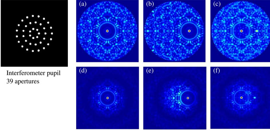
**Fig. 6.** Simulation of interferometric images for a 39 telescopes pupil. Left: pupil function. (a) IRAN on-axis PSID. (b) IRAN off-axis PSID. (c) IRAN double star image. (d) Michelson on-axis PSID. (e) Michelson off-axis PSID. (f) Michelson double star image.
