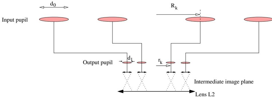
**Fig. 2.** Geometry of the interferometer. The input-to-output reduction factor of the distances between the telescopes is  $\gamma = R_k/r_k$ . The same factor for the individual pupils diameters is  $\gamma_d = d_0/d_1$
