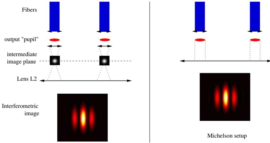
**Fig. 4.** Comparison of IRAN (left) and Michelson (right) setups for a fiber optics beam transport.
