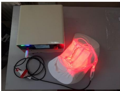
Figure 2. Complete device with medical panty, light diffuser support and laser source
