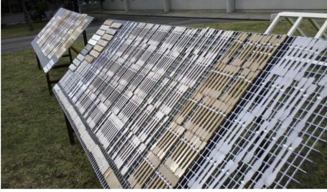
Fig. 1. Exposure racks used in this study.
