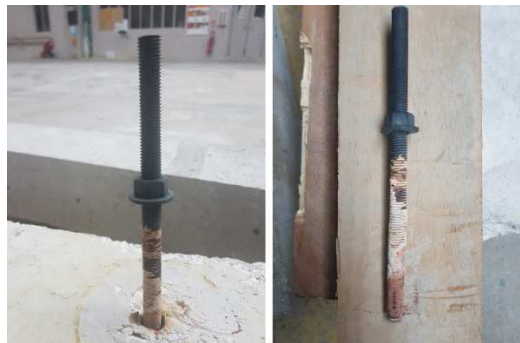
Fig. 11. Illustration of pull-out failure at the steel/resin interface of loaded bonded anchors under fire
