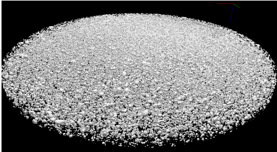
Figure 14: 3D reconstruction of pores obtained with Imorph software [36][37].
