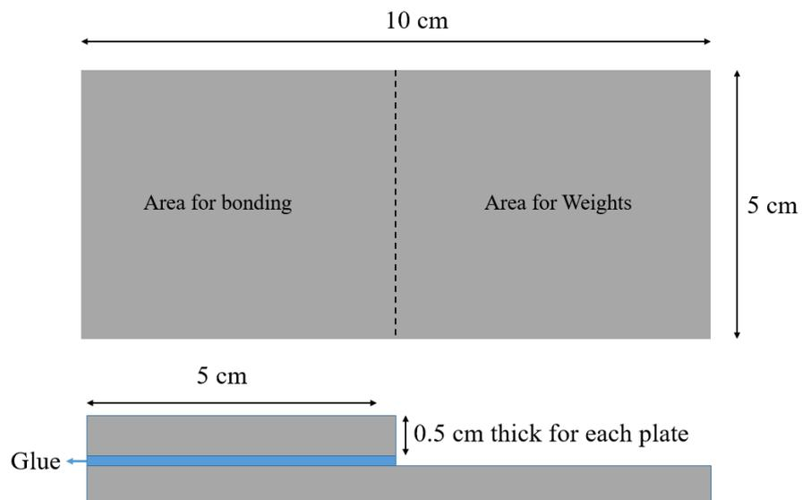
Figure 2: Top and side view of the specimen
