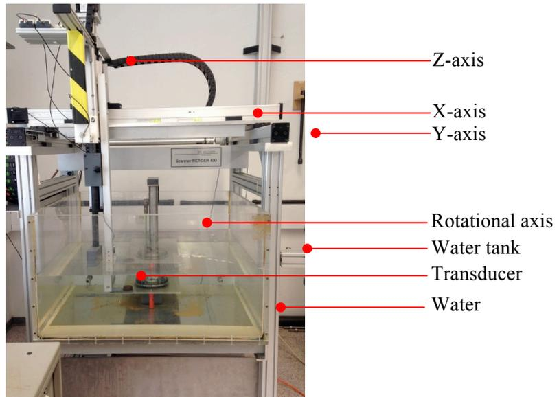
Figure 1: Ultrasonic device
