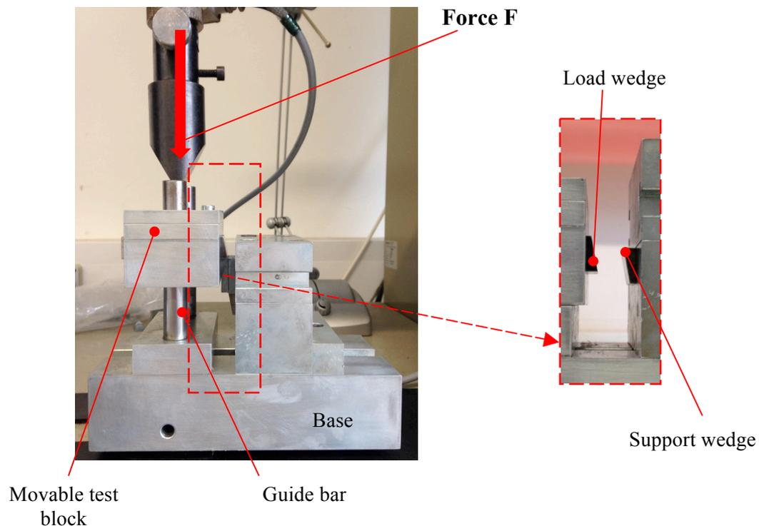
Figure 3: Shear device
