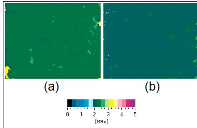
Figure 6: F-scan of (a) 5:5 Mixture (good bond), (b) 7:3 Mixture (kissing bond)
