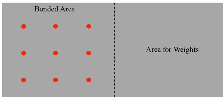
Figure 5: Inspected points (red) on bonded area of specimen
