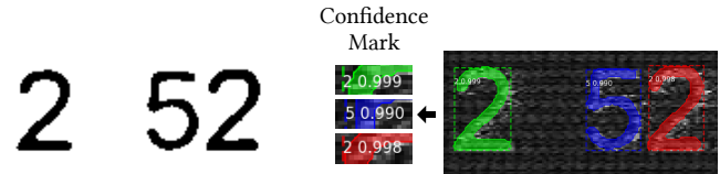
Fig. 3: The output of Mask R-CNN may be used in two ways. The segmentation can be drawn (left) and further processed by an Optical Character Recognition (OCR), or the Mask R-CNN classifier can directly infer the sample content (right) and propose some display and confidence information.
