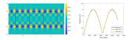
FIGURE 4. Test 1-b (barotropic Rossby wave), HCCS solver in space. The final time is t=1203 days (100 periods). The time scheme is the ERK2 time scheme with 9289 time iterations and CFL = 16, see (21). Left panel: total h at final time. Right panel: history of the relative errors for h,  $u_{\lambda}$  (zonal velocity) and  $u_{\theta}$  (meridional velocity). The three curves are almost superposed. The resolution of the Cubed-Sphere is  $6 \times 64 \times 64$ .
