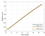
FIGURE 2. Test 1-a (barotropic EIG wave). The final time is t=13.5 days. Left panel: total height at final time. Right panel: Histories of relative errors (29-30) for the zonal velocity is  $u_{\lambda}$ , the meridional velocity  $u_{\theta}$  and the total height h. The time scheme is the ERK2 scheme with 407 time iterations and CFL = 4, see (21). The resolution of the Cubed-Sphere is  $6 \times 64 \times 64$ .
