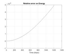
FIGURE 11. Test 1-b (barotropic Rossby wave). Mass and energy relative error (32). HCCS solver in space with ERK2 scheme time scheme with CFL = 16. The conservation accuracy is very good, even after 1203 days, (100 periods) with a level below  $5.10^{-8}$  in both cases. The Cubed-Sphere is  $6 \times 64 \times 64$ .
