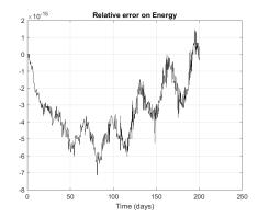
FIGURE 12. Test 2-a (baroclinic EIG wave). HCCS solver in space with the ERK2 time scheme with Courant number CFL = 5. Left panel: Mass relative error. Right panel: Energy relative error. In both case, the level is below  $5.10^{-15}$ , (machine accuracy). The Cubed-Sphere grid is  $6 \times 64 \times 64$ .
