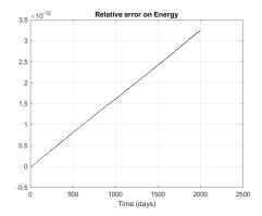
FIGURE 13. Test 2-b (baroclinic Rossby wave). HCCS solver in space with the ERK2 time scheme with Courant number CFL = 5. Left panel: history of the relative mass error. Right panel: history of the relative energy error. 1850 days represent 100 periods. The conservation error is below  $5.10^{-12}$  in both cases. The Cubed-Sphere grid is  $6 \times 64 \times 64$ .
