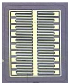
Fig.9b. Fabricated interdigitated VJFET.
