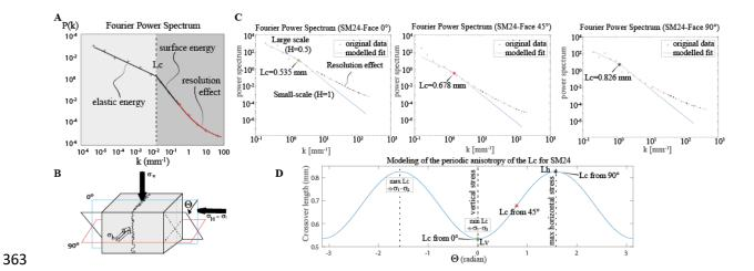
Figure 3: A – Ideal example of Fourier power spectrum applied to 1D profile of stylolite 364 roughness, showing the different expected power laws and where the crossover length sits. B – 365 366 Sketch of the cuttings through a tectonic stylolite in order to access the stylolite-plane anisotropy (after Beaudoin et al., 2016). C - Example of treatment for 3 cuts on the sample
