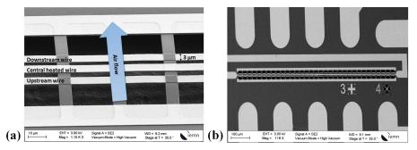
Fig. 1 (a) SEM image focused on the HTGC micro-sensor sensitive part along with legend and schematic (b) SEM image of the complete sensitive part of the HTGC micro-sensor
