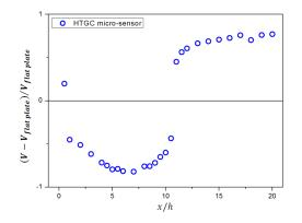
Fig. 9 Time-averaged HTGC response combining the central wire response and the lateral wires response for  $Re_h = 2.56 \times 10^4$  and for x/h going from 0.5 to 20
