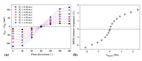
Fig. 4 (a) Voltage difference between the two lateral wires as function of the flow direction for various  $U_{\tau}$  (b) HTGC micro-sensor response to positive and negative wall shear stress
