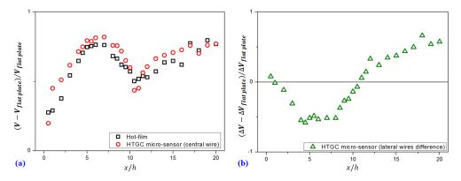
Fig. 8 (a) Time-averaged shear stress measurements with the HTGC micro-sensor central wire (circles) and the hot-film (square symbols) for  $Re_h = 2.56 \times 10^4$  and for x/h going from 0.5 to 20 (b) Time-average difference of resistance between the two lateral wires
