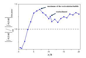
Fig. 10 Energy of voltage fluctuations downstream the rib normalized by the energy obtained in flat plate, for  $Re_h = 2.56 \times 10^4$  and for x/h going from 0.5 to 20
