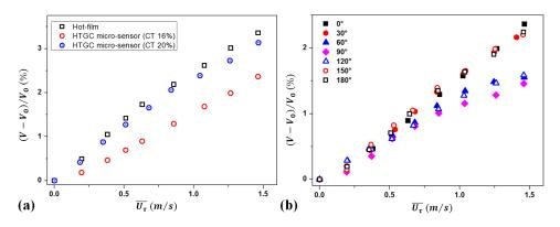
Fig. 3 (a) Calibration curves of the HTGC micro-sensor and the hot-film probe (b) Flow direction influence on the HTGC micro-sensor central wire sensitivity
