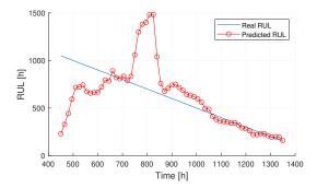
Fig. 10. RUL prediction at different moments in CC operating mode.
