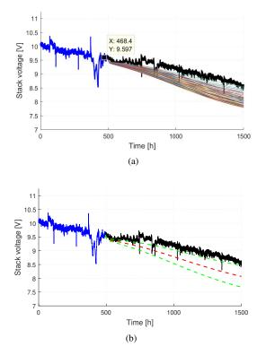
Fig. 9. Prognostic result by implementing ensemble ESN models with 1000 h prediction length. Blue line: data used for training ESN ensemble models; Black line: measured voltage evolution. (a) Prediction results of multiple models (colorful thin lines). (b) Mean predicted result (red dotted line) and CI (green dotted line).
