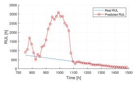
Fig. 15. RUL prediction at different moments in dynamic operating mode.
