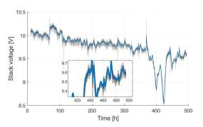
Fig. 8. Training results of ensemble ESN models. Grey line: measured stack voltage evolution; Colorful lines: estimated results from the trained ESN models.
