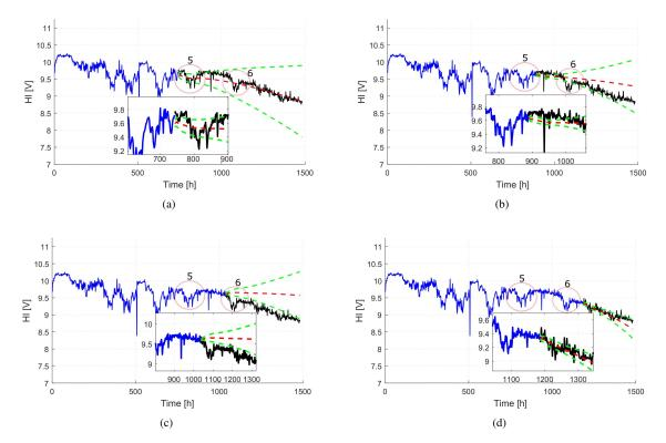
Fig. 14. Prognostic result by implementing ensemble ESN models. Blue line: data used for training ESN ensemble models; Black line: measured voltage evolution. (a) Mean predicted result (red dotted line) and CI (green dotted line) at 750 h (b) Mean predicted result and CI at 900 h (c) Mean predicted result and CI at 1050 h (d) Mean predicted result and CI at 1200 h.
