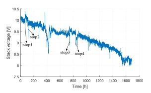
Fig. 1. Stack voltage evolution in CC experimental setting
