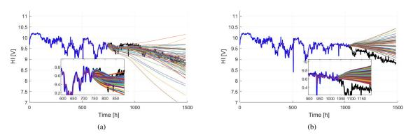
Fig. 13. Prediction results by implementing multiple ESN models. Blue line: data used for training ESN ensemble models; Black line: measured voltage evolution. Colorful thin lines: predicted results of multiple models. (a) Prediction result at 750 h (b) Prediction results at 1050 h.
