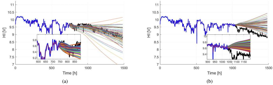
Fig. 13. Prediction results by implementing multiple ESN models. Blue line: data used for training ESN ensemble models; Black line: measured voltage evolution. Colorful thin lines: predicted results of multiple models. (a) Prediction result at 750 h (b) Prediction results at 1050 h.
