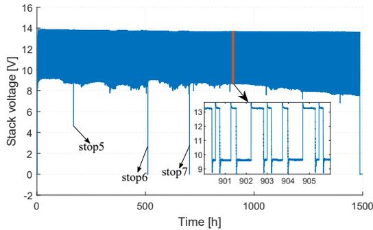
Fig. 3. Stack voltage evolution in dynamic experimental setting
