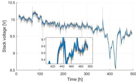
Fig. 8. Training results of ensemble ESN models. Grey line: measured stack voltage evolution; Colorful lines: estimated results from the trained ESN models.
