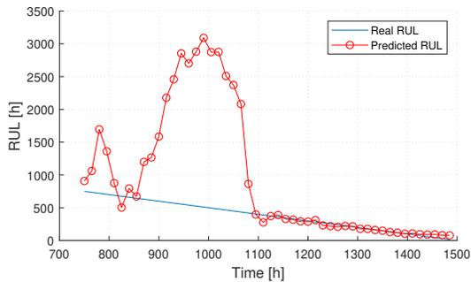
Fig. 15. RUL prediction at different moments in dynamic operating mode.
