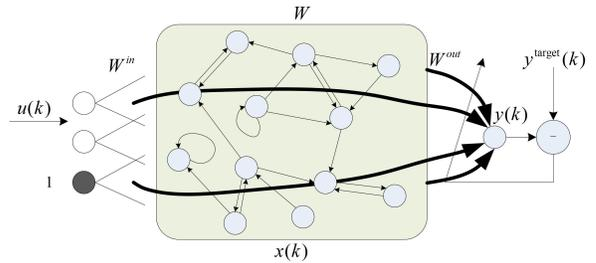
Fig. 5. Illustration of the basic ESN structure, adapted from [24].
