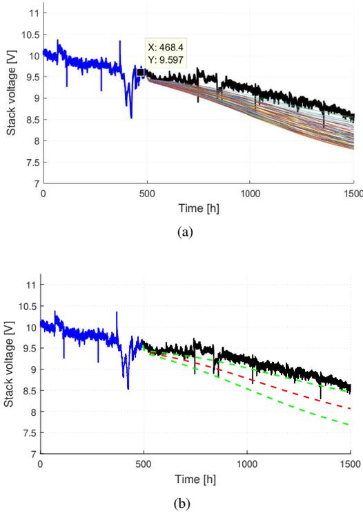
Fig. 9. Prognostic result by implementing ensemble ESN models with 1000 h prediction length. Blue line: data used for training ESN ensemble models; Black line: measured voltage evolution. (a) Prediction results of multiple models (colorful thin lines). (b) Mean predicted result (red dotted line) and CI (green dotted line).
