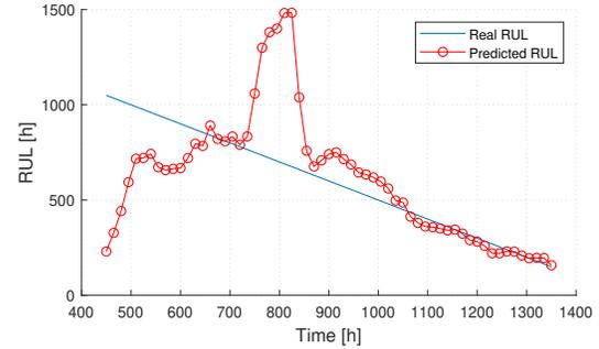
Fig. 10. RUL prediction at different moments in CC operating mode.
