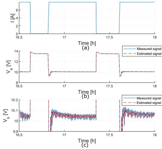
Fig. 11. Model identification performance in one data segment.
