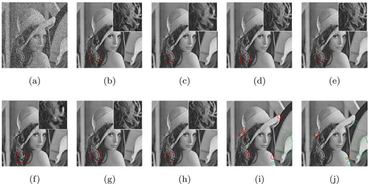
Fig. 16. Denoising results for Lena image (noise density is 30%). (a) Corrupted image. (b) ASWM. (c) ROR-NLM. (d) BDND. (e) IBNDND. (f) WCSR. (g) ASMF-DBER I. (h) ASMF-DBER II. (i) Colored detection results of ASMF-DBER I. (j) Colored detection results of ASMF-DBER II. (For interpretation of the references to colour in this figure legend, the reader is referred to the web version of this article.)
