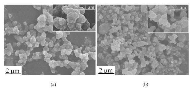
Figure 2: FE-SEM micrograph of the (a) HA and (b) β-TCP starting powders. Insets: higher magnification micrographs.
