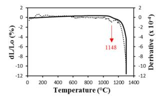
Figure 6: Linear shrinkage (solid line) and derivatives curves (dashed lines) versus temperature of the BCP1 single bar. One peak, corresponding to the partial decomposition of CDA into  $\beta$ -TCP, is identified with the corresponding temperature.
