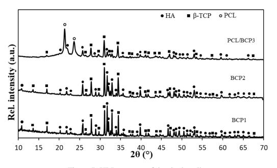
Figure 7: XRD patterns of the single pellets
