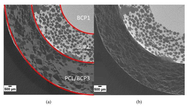
Figure 12: Slice of 3D X-Ray Tomography images of a scaffold (a) before and (b) after immersion for 17 days in TRIS. The ceramic phase has a larger absorption of X-ray as compared to the polymer and appears brighter.
