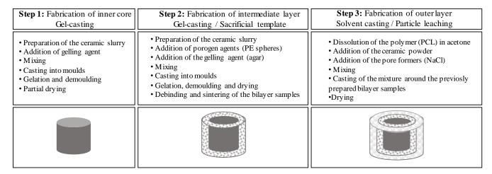
Fig. 1: Schematic diagram illustrating the main steps of the fabrication of the graded scaffold. In the bottom part, the specimens at the different steps of the process are graphically shown.
