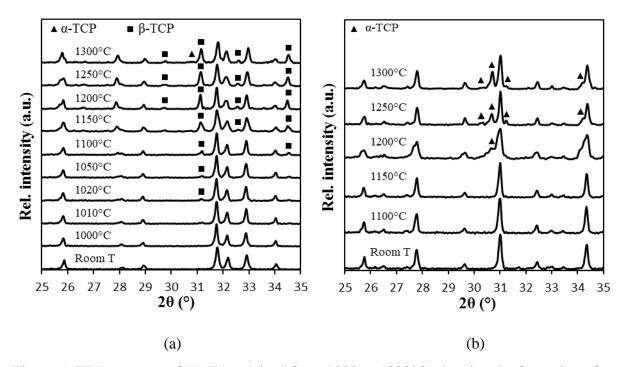
Figure 5: XRD patterns of (a) HA calcined from 1000 to 1300°C, showing the formation of  $\alpha$ -and  $\beta$ -TCP (the non-indexed peaks correspond to HA) and (b)  $\beta$ -TCP calcined from 1100 to 1300°C showing its conversion into  $\alpha$ -TCP (the non-indexed peaks correspond to  $\beta$ -TCP)
