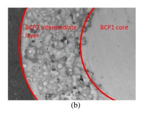
Figure 9: (a) Digital picture (bottom part) and schematic illustration (upper part) of the three-layer scaffold with BCP1, BCP2 and PCL/BCP3 layers from the centre to the periphery and (b) stereomicroscope image of a polished surface evidencing the interface between the BCP1 and BCP2 layers
