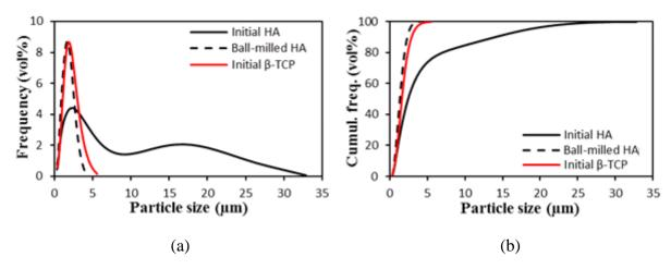
Figure 3: Frequency (a) and cumulative frequency (b) distributions of as-received and ball-milled HA and of as-received  $\beta$ -TCP.
