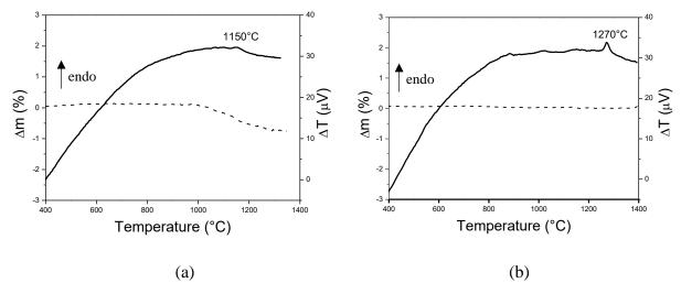
Figure 4: DTA-TG curves of (a) HA and (b)  $\beta$ -TCP powders. The two main peaks with the corresponding temperatures are identified.
