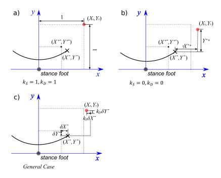
Fig. 3: Influence of  $k_S$  and  $k_D$  on the foot locations. a) Step length and width are fixed; b) The initial CoM position error is nullified; c) The general case. The black and the red dots represent respectively the stance feet during the current and the next steps. The curved line represents the CoM trajectory, and the cross the CoM position at the end of the current step.
