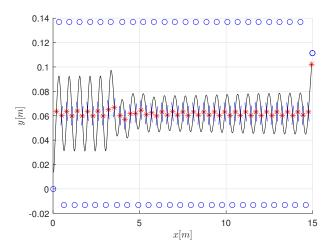
Fig. 17: The projection of the VLIP motion in horizontal plane for 50 steps when  $k_S = 0, k_D = 1$ . The black curves represent the CoM evolution, the blue circles represent the stance foot placements, and the blue lines represent the swiching manifold.
