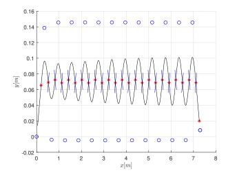
Fig. 8: The projection of the VLIP motion in horizontal plane for 25 steps when  $k_S = 0, k_D = 0$ . The black curves represent the CoM evolution, the blue circles represent the stance foot placements, and the blue lines represent the swiching manifold.
