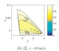
Fig. 14: Maximal norm of eigenvalues for different  $\dot{z}_m^d$  as a function of C and  $k_v$  when  $k_S=0, k_D=1$ .
