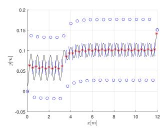
Fig. 15: The projection of the VLIP motion in horizontal plane for 40 steps when  $k_S = 0, k_D = 0$ . The black curves represent the CoM evolution, the blue circles represent the stance foot placements, and the blue lines represent the swiching manifold.
