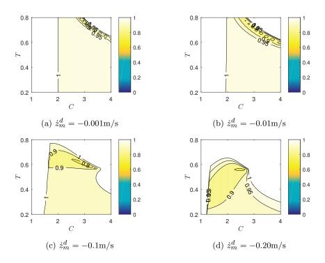
Fig. 7: Maximal norm of eigenvalues for different  $\dot{z}_m^d$  when  $k_S=0, k_D=1$ . Contrary to the white areas, the colored areas indicate self-stabilization condition.
