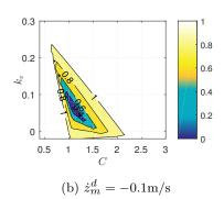
Fig. 13: Maximal norm of eigenvalues for different  $\dot{z}_m^d$  as a function of C and  $k_v$  when  $k_S=0, k_D=0$ .
