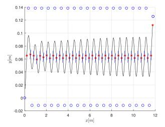
Fig. 10: The projection of the VLIP motion in horizontal plane for 40 steps when  $k_S = 0, k_D = 1$ . The black curves represent the CoM evolution, the blue circles represent the stance foot placements, and the blue lines represent the swiching manifold.
