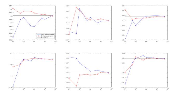
Figure 1: The Sobol g-function model (37). Convergence of both methods when N increases. The sixth first-order Sobol indices have been represented from left to right and up to bottom. Several sample sizes have been considered:  $N=100,\ 500,\ 1000,\ 5000,\ 10000,\ 50000,\ 100000,\ 100000,\ and\ 500000$  for the Pick-Freeze estimation procedure and correspondingly (p+1)N for the estimation procedure proposed in [7]. The x-axis is in logarithmic scale.
