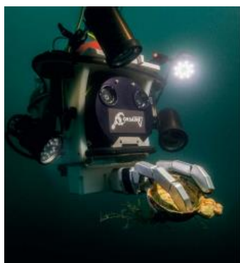
Fig. 1: The teleoperated ROV with Technoconcept gripper © DRASSM
