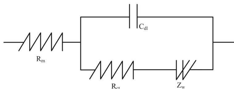
**Fig. 8** Equivalent circuit of FC [55]
