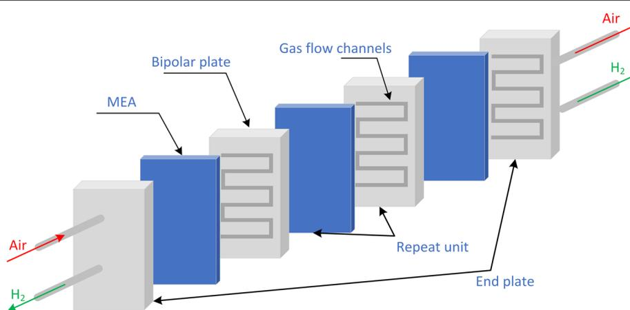
**Fig. 3** Schematic of PEMFC stack
