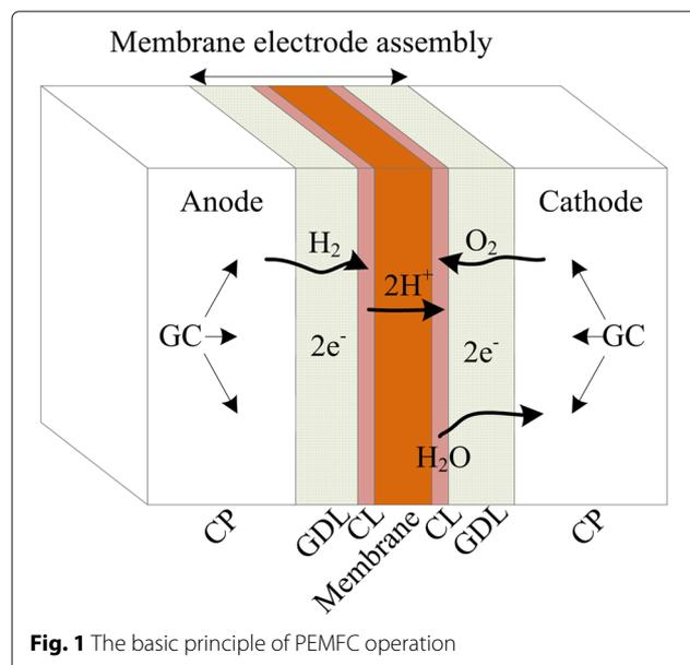
**Fig. 1** The basic principle of PEMFC operation
