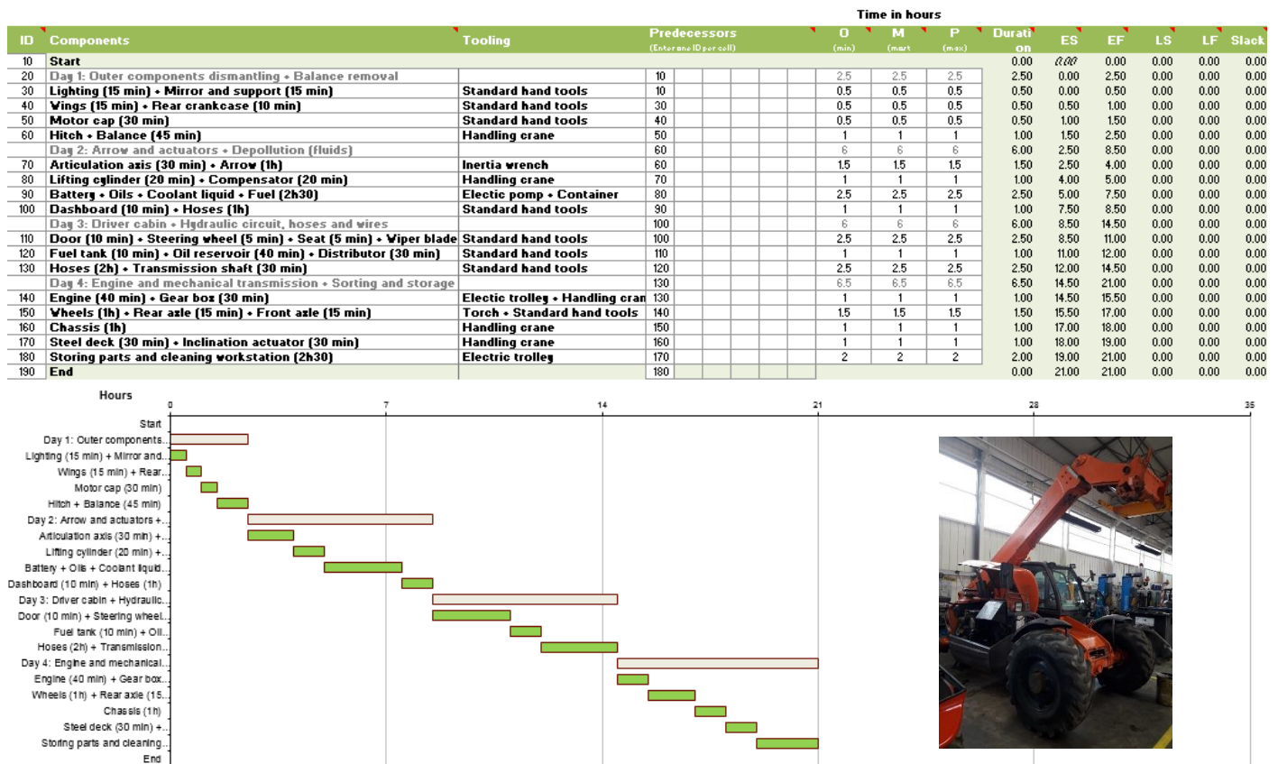
Figure B5 – Gantt chart of the newly validated dismantling process after a second dismantling test
