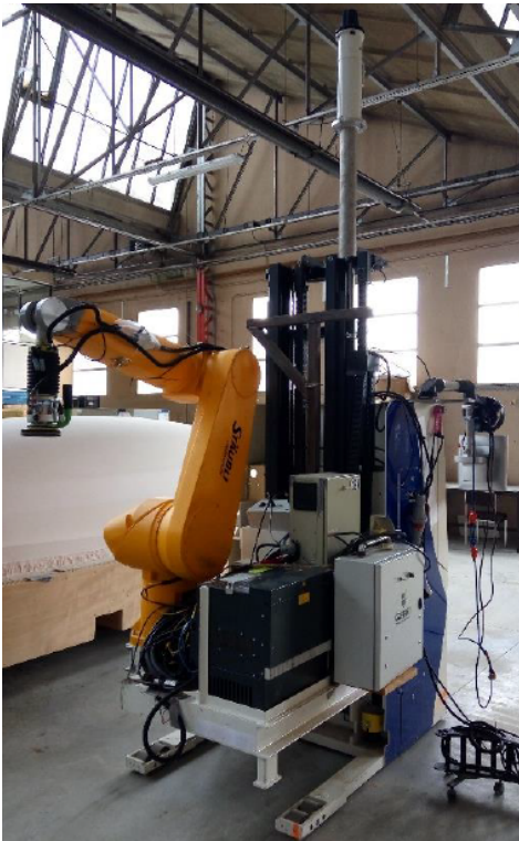
Fig. 1. Mobile Robot developed to perform sanding application : it includes an Automated Guided Vehicle, An industrial Robot Staubli RX160L and an active compliant tools for sanding
