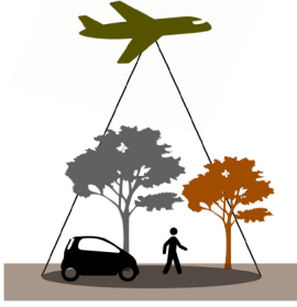
Fig. 1. An airborne MSL system can capture multiple objects per pixel and discriminate their materials. The multidepth capability enables the recovery of information from photons reflected off different branches of the trees, ground, pedestrians or even from the interior of a car (i.e., photons which propagated across the windshield) at an intra-pixel level. Moreover, the multispectral information allows us to discriminate different properties of the materials of each 3-D object (e.g., the leaves and trunk of a tree).
