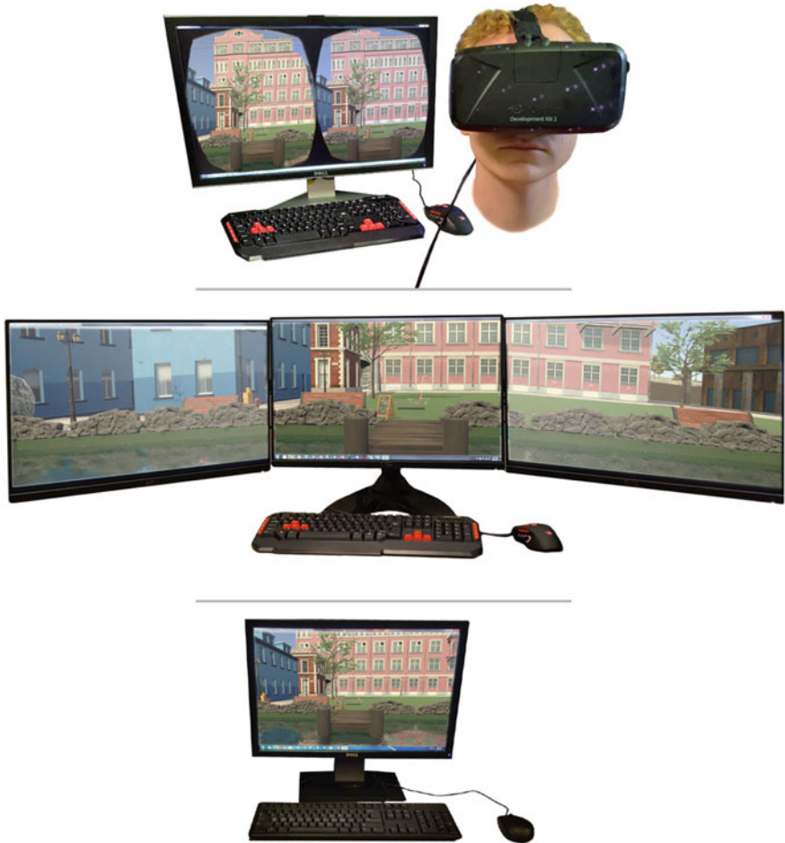
Fig. 7.15 Different levels of immersion, with immersiveness increasing from top to bottom. Increased immersion is supported by a combination of an increased field of view and the use of an egocentrically fixed rather than an allocentrically fixed reference frame. Based on Oprean et al. (2017) with the original author's permission
